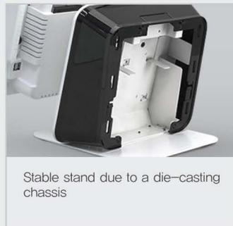
Stable stand due to a die-casting chassis
